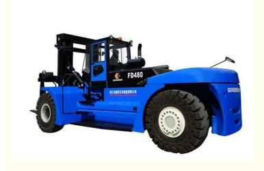
THE OVERALL WIDTH OF THE HEAVY DUTY DRIVE AXLE (4.22M OVER TYRES), WITH ENHANCED SPINDLES WITH DOUBLE REDUCTION PROVIDES FIRMNESS AND WEAR WHEN HANDLING THE HEAVIEST LOADS
